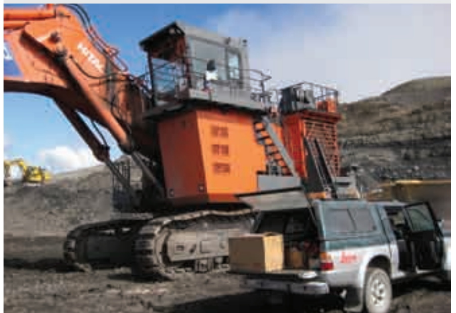
Much of the installation work was completed 'in pit', including this Leica DigNav JS system on a Hitachi 1900 (190 tonne) excavator.
